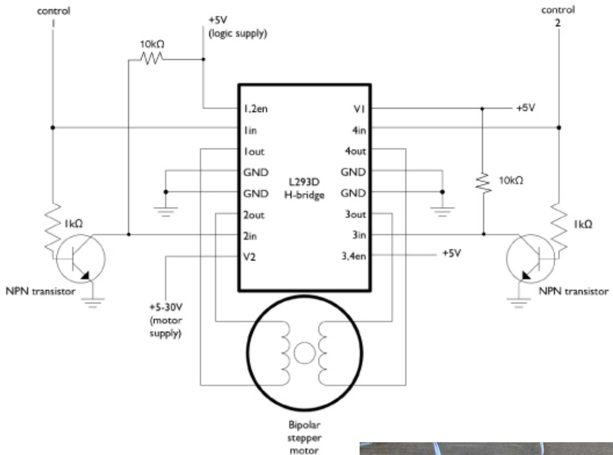
The motors are wired according to the diagram above. This allows the motors to be controlled by two pins on the arduino. Using the stepper library the arduino can generate the signal needed to turn the motors one step at a time. This method works, but it was very brute force. There are far better methods of controlling steppers, including chips designed to do so.
