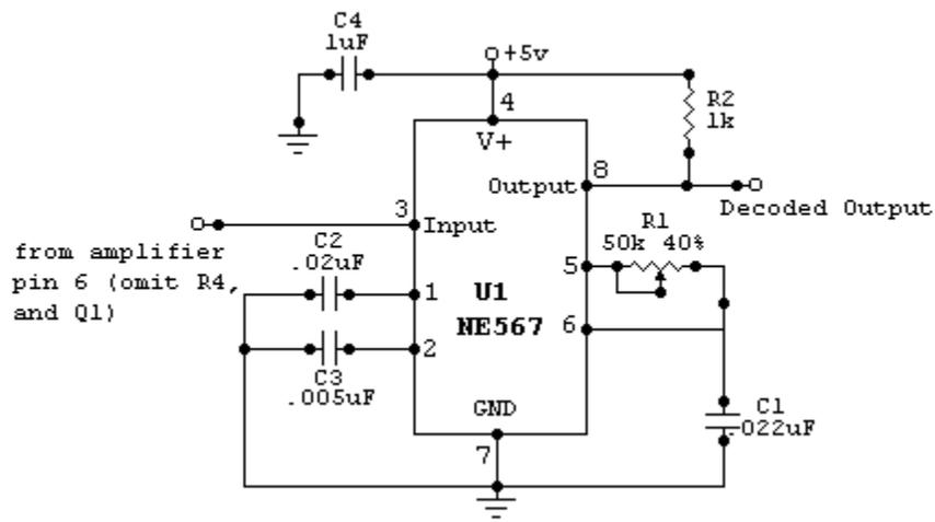
The sound sensing circuit is wired according to this diagram and the potentiometer at pins 5 and 6 should be set to around 20k, this puts the sensor in a range that responds to ambient room noise.
