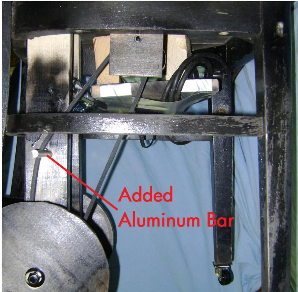
**Figure 6: Belt Tightening Solution**
