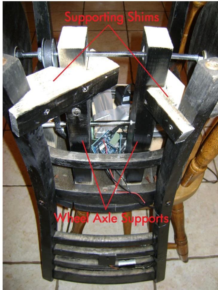
**Figure 2: Wheel Axle Support Assembly**
