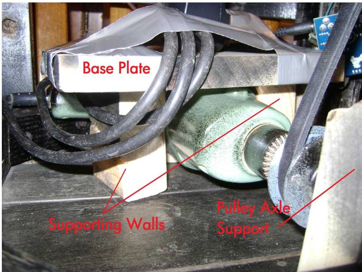
**Figure 1: Base Plate Assembly**
